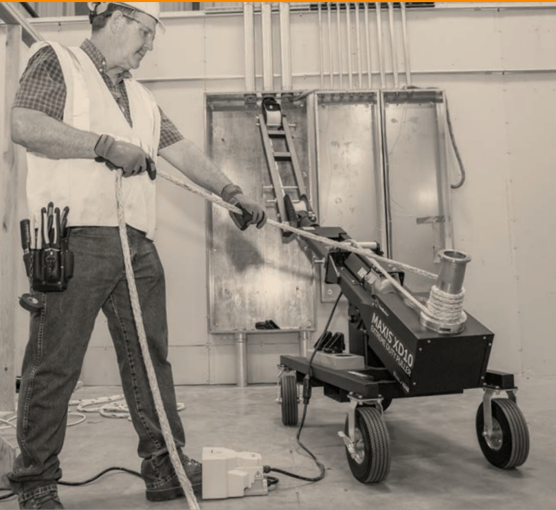
YR01889 616 6,000LB CABLE PULLER WITH MILWAUKEE MOTOR ON CART PAGE 4
