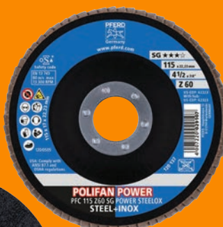
PFE62222 Flap Disc, 4-1/2" x 7/8, Z SG POWER STEELOX, 40 Grit, T29, Conical, Zirconia
